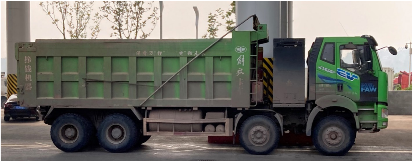
A battery swapping heavy truck with the battery mounted behind the cabin.
