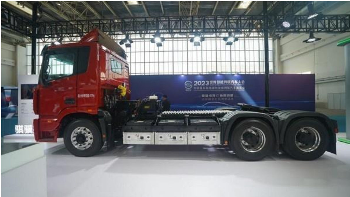
Figure 10. Aulton's second generation battery-swapping solution for trucks. Source: Xianning News Network China Youth Network.
