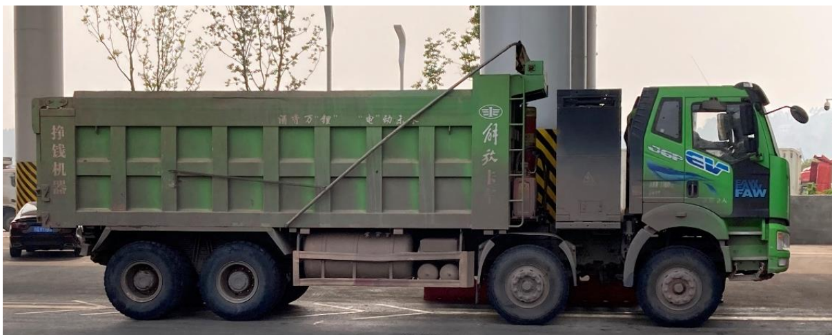
Figure 74. A battery-swapping heavy truck with the battery mounted behind the cabin.
