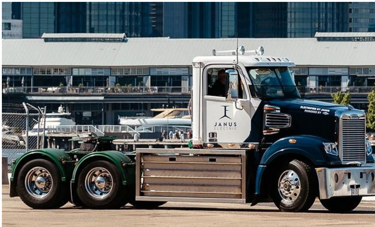
Figure 28. Janus Electric modified truck with swappable batteries from the side of the truck. Source: https://www.januselectric.com.au/ .
