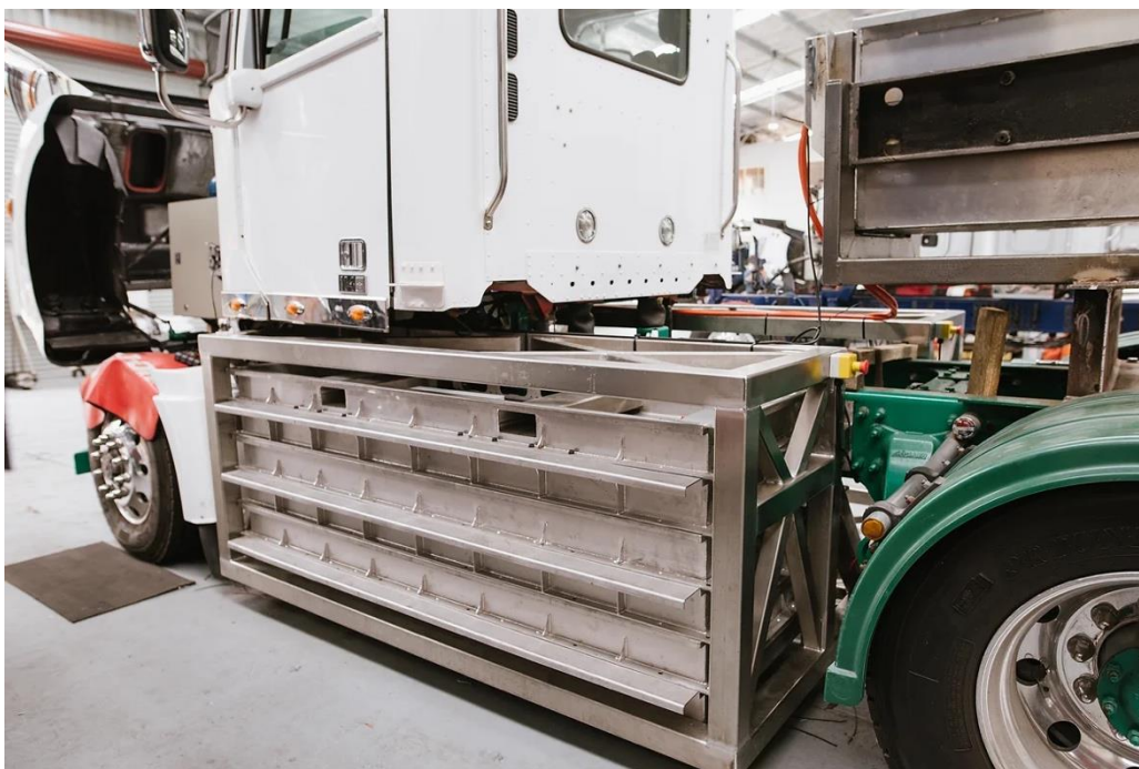
Figure 30. Janus Electric side-mounted swappable battery for heavy trucks. Source: https://cleantechnica.com/2023/03/06/truck-stops-are-very-big-in-america-could-battery-swapping-be-an-option-for-charging-all-those-trucks/ .
