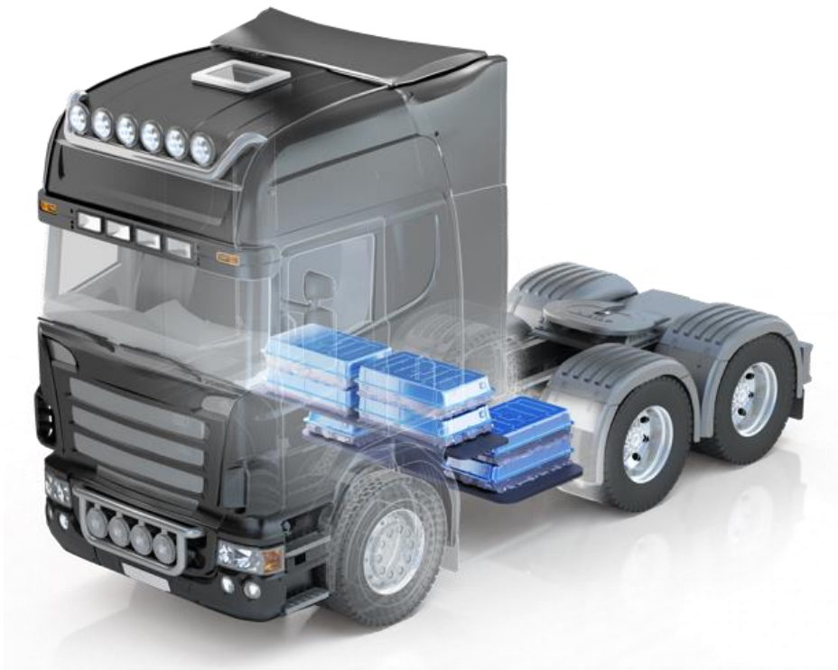
Figure 7. CATL Qiji chassis battery-swapping solution for EHTs. . Source: https://www.catl.com/en/solution/commercialEV/ .
