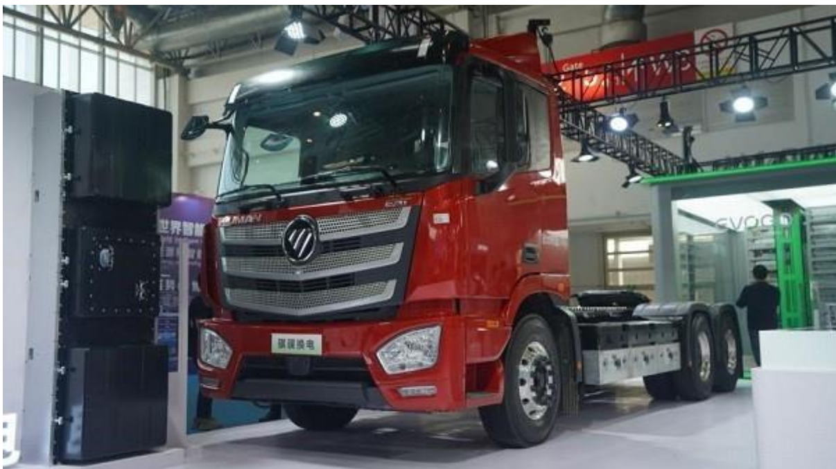
Figure 12. Aulton's second generation battery-swapping solution for trucks. Source: Xianning News Network China Youth Network.
