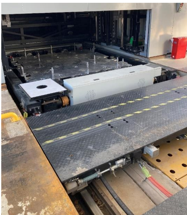
Figure 75. Swapping station DeepWay trucks, swapping from below.
