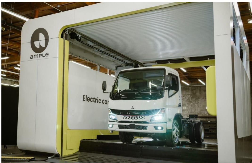
Figure 25. Ample and Mitsubishi Fuso battery-swapping station for trucks. Source: https://cleantechnica.com/2023/07/26/battery-swapping-for-large-trucks-is-this-the-way-to-go/ .
