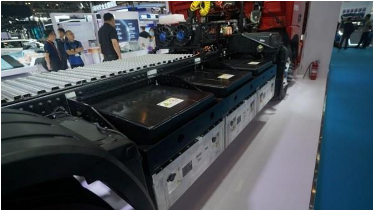
Figure 11. Aulton's second generation battery-swapping solution for trucks. Source: Xianning News Network China Youth Network.
