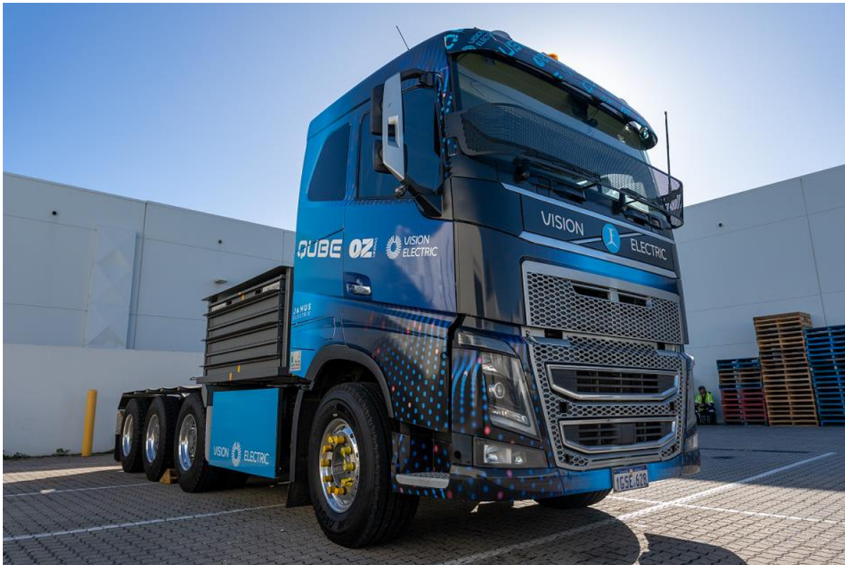
Figure 31. Janus Electric modified Volvo FH16 with battery-swapping solution. Source: https://chargedevs.com/newswire/who-says-heavy-duty-evs-wont-work-170-tonne-620-kwh-battery-electric-truck-hits-the-road-in-australia/ .
