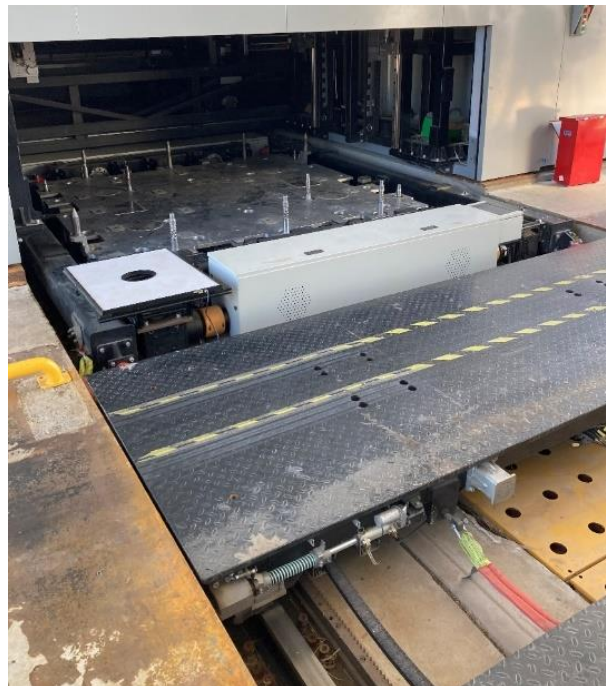
Picture: Swapping station DeepWay trucks, swapping from below
