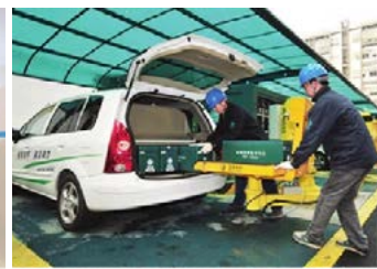
Figure 14: Rear battery mount
