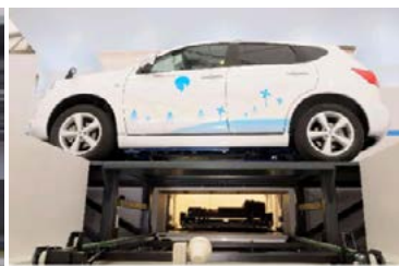
Figure 13: Bottom battery mount
