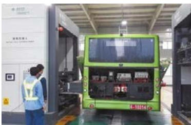
Figure 12: Side battery mount
