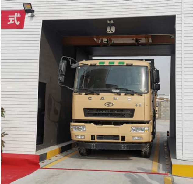
Figure 31: A CAMC EHT being served at the battery-swapping station in Zhengzhou, Henan province.
