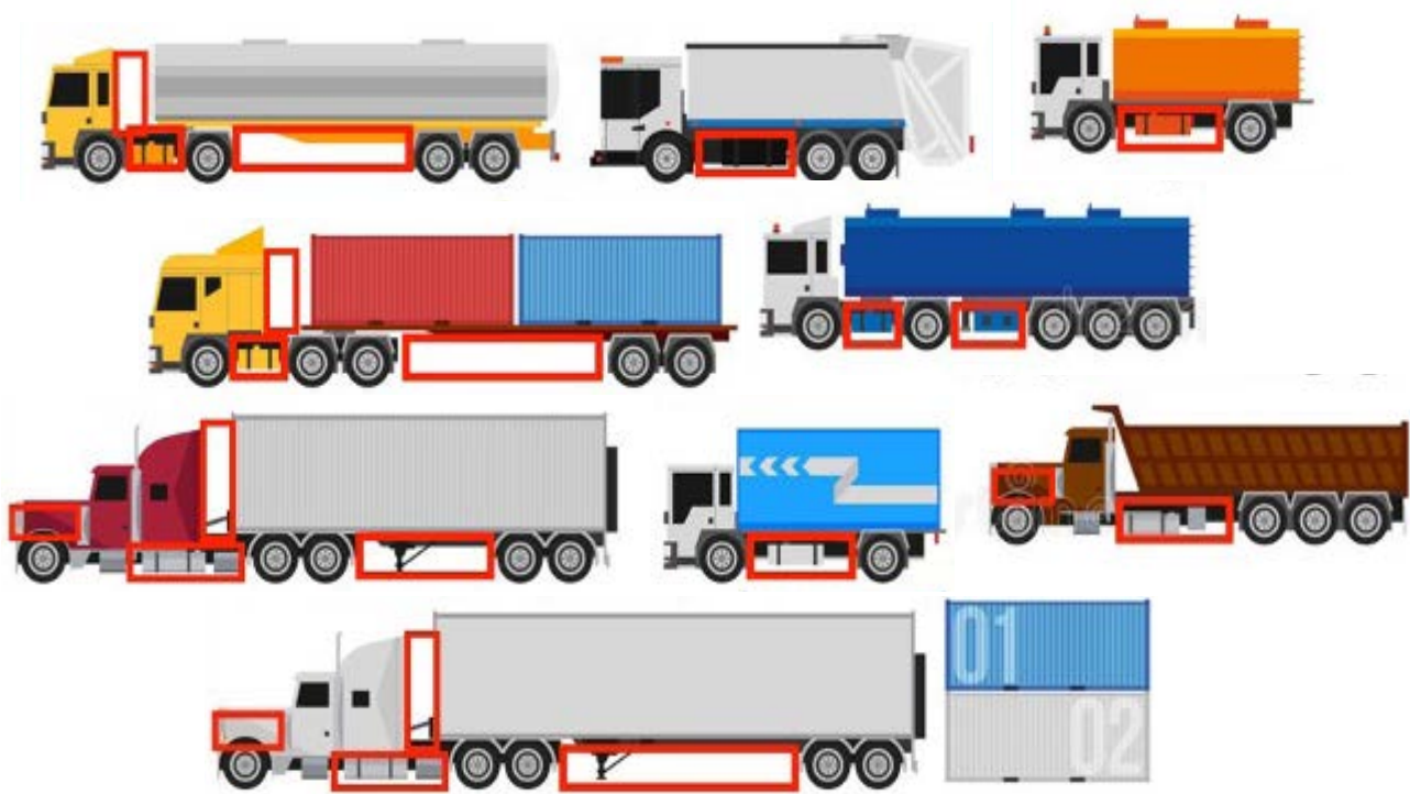
Figure 8: Battery-swapping positions on a truck.
