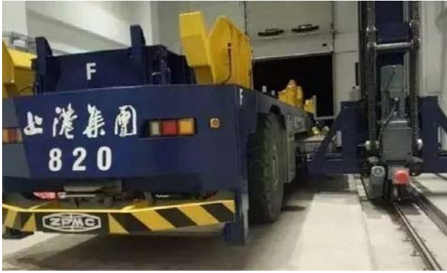
Figure 34: AGV battery-swapping solution at Yangshan Port, Shanghai.
